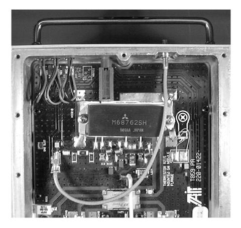
Figure 3.4 T859 Front RF Input Coax Routing
