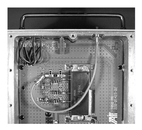
Figure 3.3 T858 Front RF Input Coax Routing
